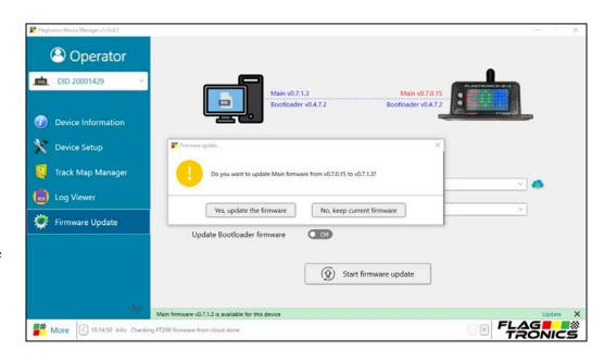
specific firmware version and are prompted to update the main firmware, click **No, keep current firmware** and then select the organization- specific firmware from the **Update Main Firmware** dropdown. For example, you can select "SCCA v0.7.1.8" or other organization-based firmware versions.
