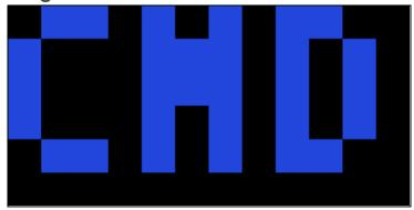
When the device is turned ON in an area with an active Flagtronics network, but the network is in 'sleep' mode, the LED screen will display 'CMD,' indicating that it is waiting for a flag command.
